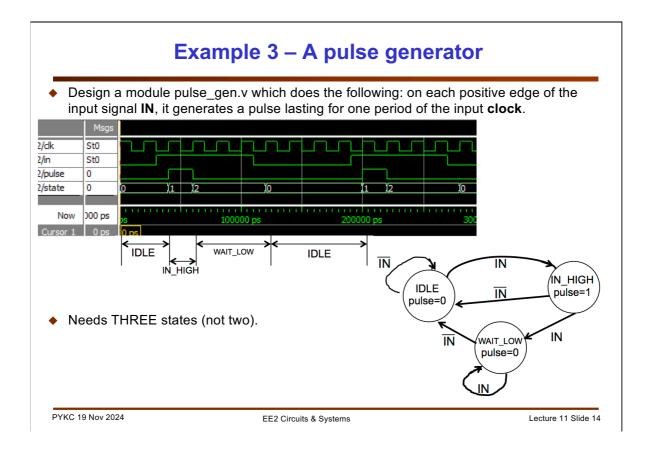
Let us now consider another example, which will appear in the Lab Experiment later. You are required to design a pulse generator circuit that, on the positive edge of the input **IN**, a pulse lasting for one clock period is produced.
