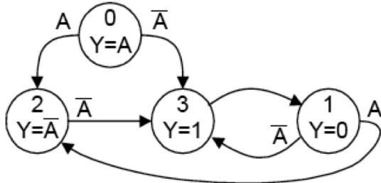
In order to make the state diagram less cluttered, you can omit the self transition arrows. Therefore the rule is that a state machine stays in its current state unless the conditions of an exiting arrow is satisfied.
