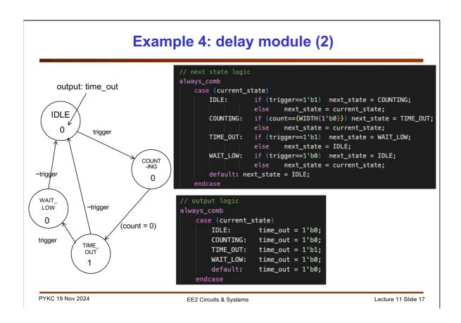
Here is the implementation. Note how the counter value is used in the state transition logic.
