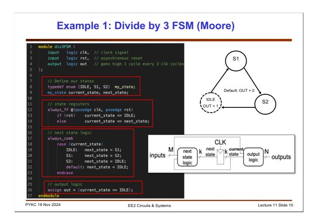
Here is a very simple three states FSM. The intial state is the IDLE state (here shown in dotted lines). The purpose of this machine is to divide clock signal by three – out goes high for one cycle every three.
